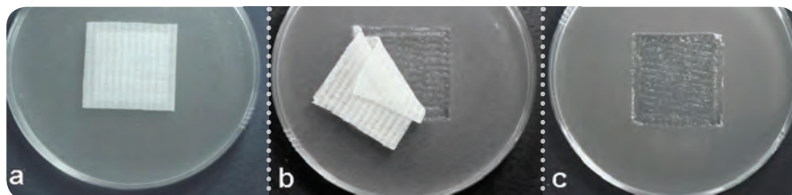
Figure 2. Preparation of indented agar model. A: gauze fixed within agar; B: gauze being removed; C: graduated indentation, showing an irregular agar surface.
