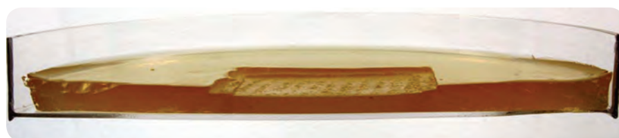
Figure 3. Cross-section of the graduated indentation (~2–3mm deep) and irregular surface.
