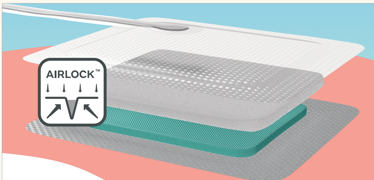
Figure 2. AIR-LOCK™ technology layer of PICO™ sNPWT (© 2023 Smith+Nephew)
