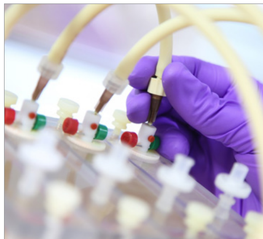
Figure 4. Image of Drip Flow Reactor. This is used to reproduce biofilms on glass coupons under defined conditions suitable for efficacy testing. The biofilms represent generalised situations where biofilm exists at the air/liquid interface with a continuous flow of nutrients under low fluid shear
