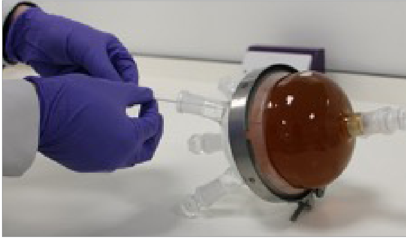
Figure 1. Bacterial barrier test model. A wound dressing is sandwiched between two sterile glass hemispheres. The wound contact surface of the dressing is challenged with a bacteria-inoculated suspension such as Pseudomonas aeruginosa . The outer (dry) surface of the dressing is swabbed and cultured daily to determine whether bacteria have penetrated the dressing, and if so, at what time point
