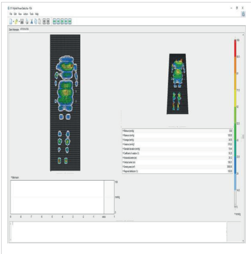
Figure 1. Typical pressure map showing distribution of pressure while supine on the static powered hybrid
